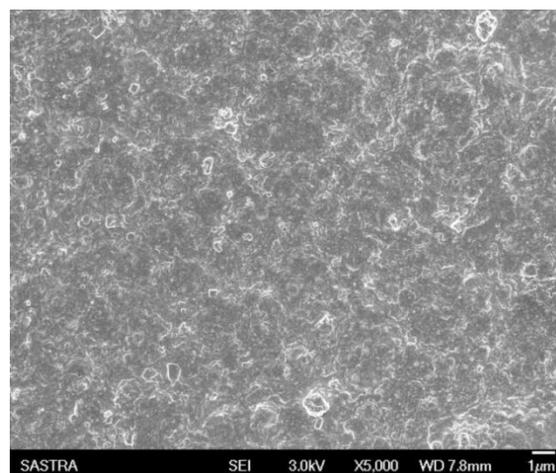
Figure 4. SEM image of nickel-tungsten (50  $\mu\text{m}$ ) coating
