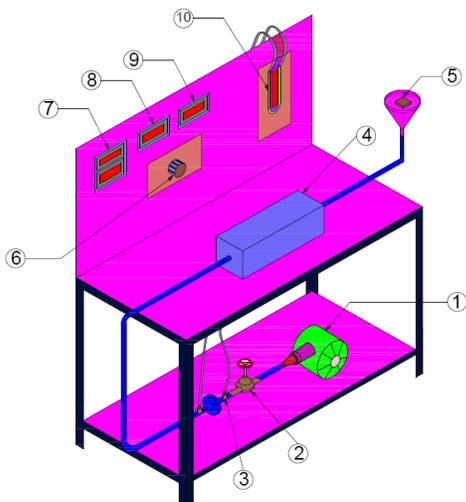
Figure 2. Schematic diagram of the experimental set up to study the convective heat transfer behaviour of the coatings [Not to scale] 1. Blower 2. Foot Valve. 3. Orifice meter. 4. Heating Section 5. Specimen. 6. Variac, 7. Temperature indicator. 8. Voltmeter. 9. Ammeter. 10. Manometer
