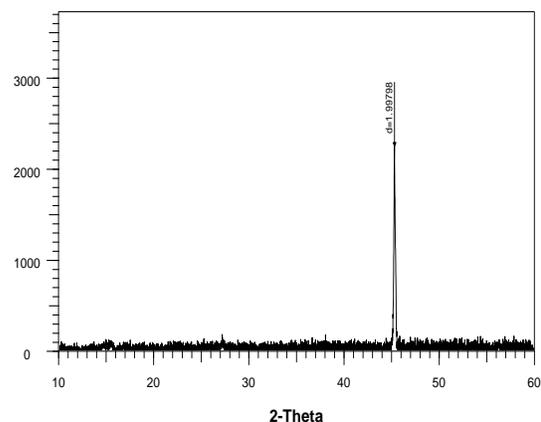
Figure 3. XRD pattern of Nickel tungsten (50  $\mu\text{m}$ ) coating
