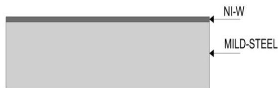
Figure 1. Schematic diagram of Nickel-Tungsten electro-deposit over mild steel sub strate
