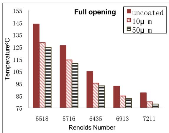
Figure 8 Temperature Vs Reynolds number
