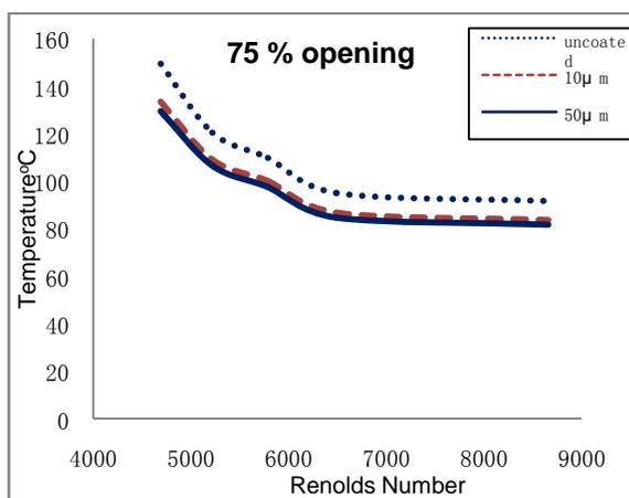
Figure 10. Temperature Vs Reynolds number
