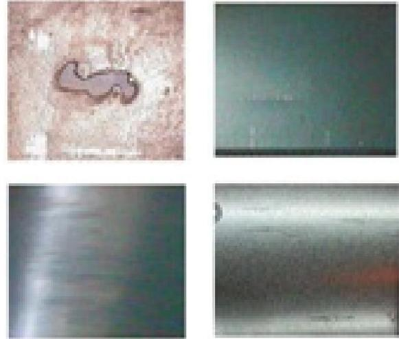
Hole, Wrinkle, Corrosion, Scrape (From Top to Bottom)
