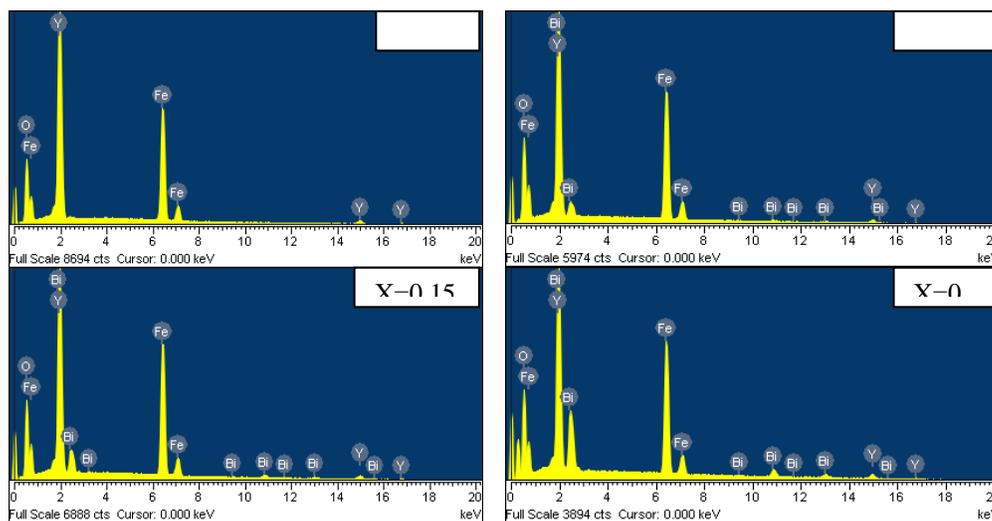
Fig. 2: XRF pattern of  $\text{Y}_{1-x}\text{Bi}_x\text{FeO}_3$  powders for  $x=0, 0.1, 0.15$  and  $0.2$ .
