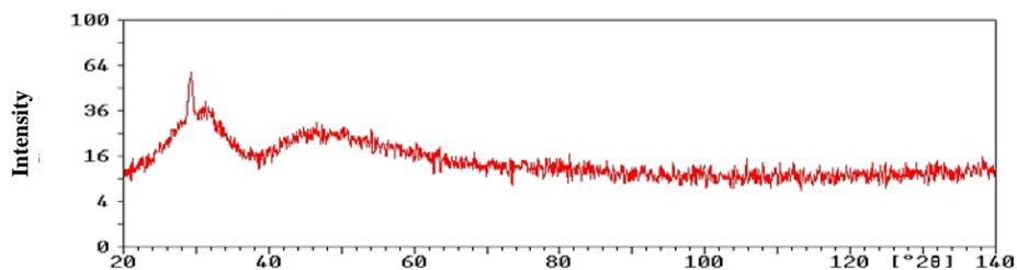
Fig.4. XRD diffraction pattern of  $Y_{0.8}Bi_{0.2}FeO_3$  film
