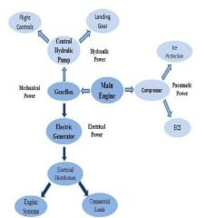
Figure 4.2 Schematic conventional aircraft power distribution system.
