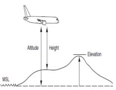
Figure 6.7 Elevation, altitude and height
