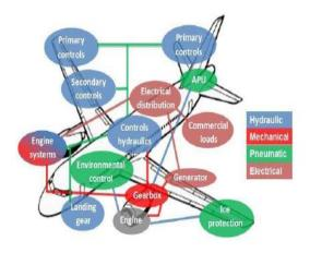
Figure 4.1 Schematic conventional aircraft
