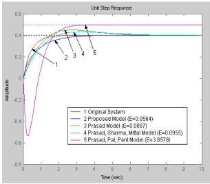
Figure 3: Unit step response curves for  $G_{12}(s)$
