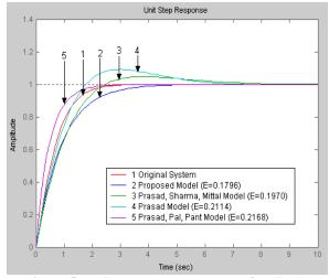
Figure 5: Unit step response curves for  $G_{22}(s)$
