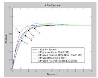
**Figure 2:** Unit step response curves for  $G_{11}(s)$
