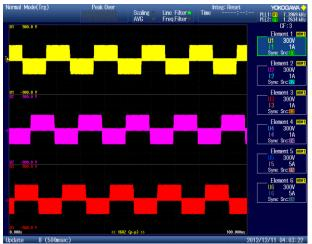
Figure 8. SPWM; M.I.=0.8; Line to Line Voltage
