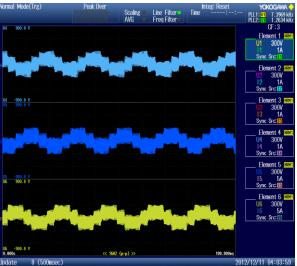
Figure 9. SPWM; M.I.=0.8; Line to Neutral Voltage
