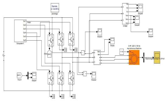
Figure 2. Matlab Simulation model of the Inverter circuit
