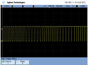
Figure 7. DSO Output of RFPWM
