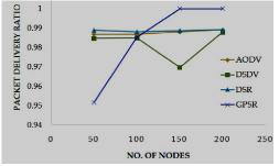
Figure 8.Comparison of Packet Deliver Ratio of GPSR with traditional protocols
