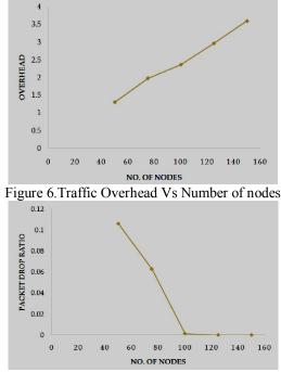
Figure 7.Packet Drop Ratio Vs Number of nodes
