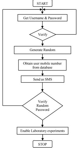
Figure 1. Flowchart Representation of Authentication through Random Number
