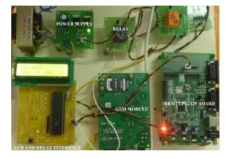
Figure 11. Complete hardware module with GSM modem and Interface circuit module
