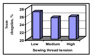
Figure 7: Effect of sewing thread tension on the seam elongation.
