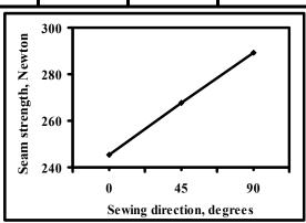
Figure 4: Effect of sewing direction on the seam tensile strength.
