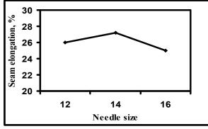
Figure 5: Effect of needle size on the seam elongation.
