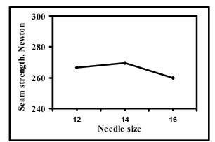
Figure 1: Effect of needle size on the seam tensile strength.
