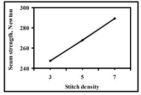
Figure 2: Effect of stitch density on the seam tensile strength
