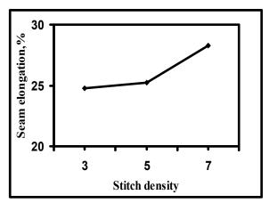
Figure 6: Effect of stitch density on the seam elongation.
