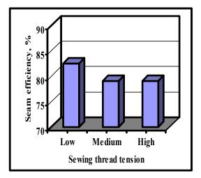
Figure 11: Effect of sewing thread tension on the seam efficiency.
