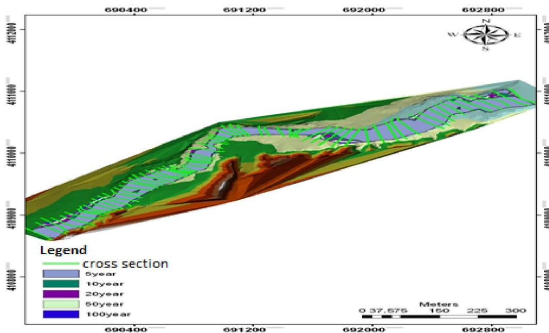
Figure 5: Flood zoning of a part of Ay-Doghmarsh River using HEC-RAS model and ARC GIS software
