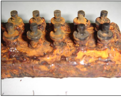
Fig. 12 The appearance of stainless wire after 2000 hours salt spray test
