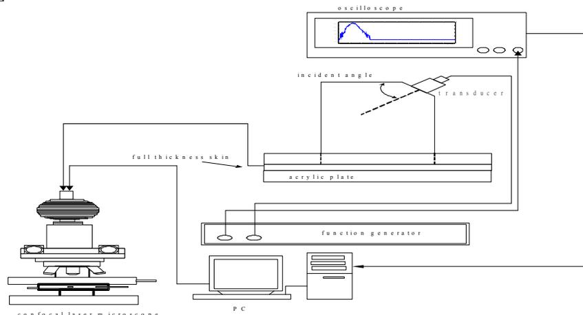
**Figure 2.** Schematic diagram of the isonation and measurement apparatus used in the exposure experiments [11].
