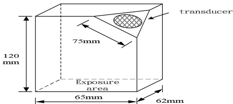
**Figure 1.** Dimensions of the exposure wedge. The orientation of the transducer is fixed in the corner of the chamber [11].
