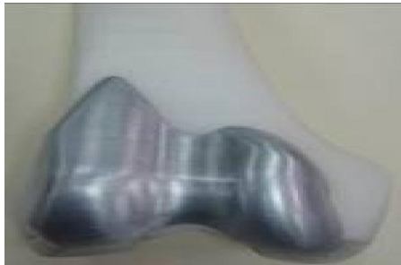
Figure 13. Assembling test of the machined femoral component and the cut femur.
