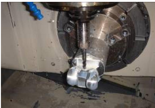
Figure 12. The five-axis machining of femoral component on five-axis machine tool.
