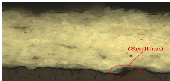
Figure 7(i) ZrO 2 coating with high pressure air cleaning, magnification 200X.
