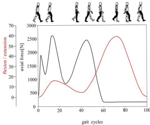
Figure 3: Variation of the axial force with gait cycle.
