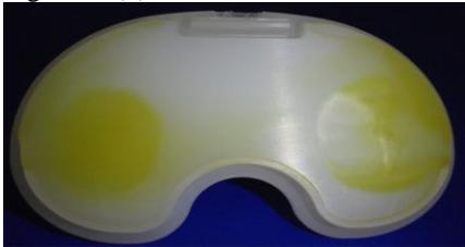
Figure 13 Insert backside surface after test of 5,000,000 cycles.
