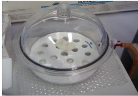
Figure 10 Vacuum drying system: YSC DP-40V
