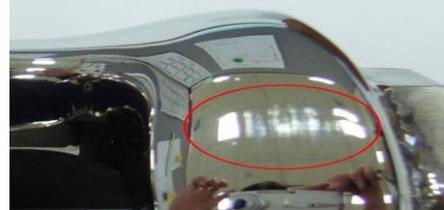
Figure 11(b) Femoral component: after test of 5,000,000 cycles.
