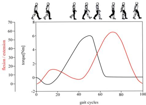
Figure 5: Variation of the tibial torque with gait cycle.
