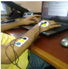
Figure 3(a): Placement of sEMG electrodes on hand ( musculilumbricalesmanus ) and forearm ( extensor carpi radialis )
