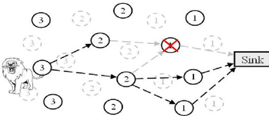
Figure 8. Sensor network continues to forward packets when some nodes fail
