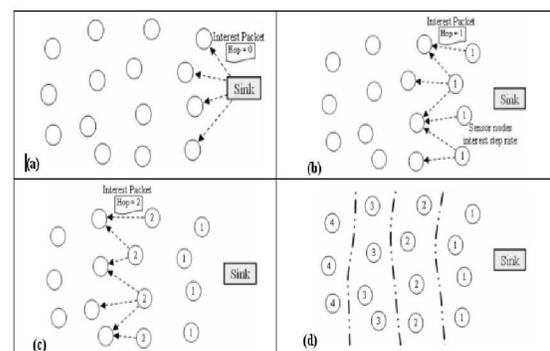
Figure 1. Different steps of first phase of EEAR to detect layers
