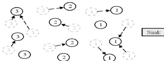
Figure 6. Packet routing in sleeping nodes
