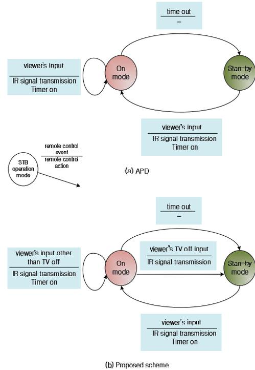
Figure 2 State diagrams of STB operation based on viewer’s remote control input event for APD and for the proposed scheme
