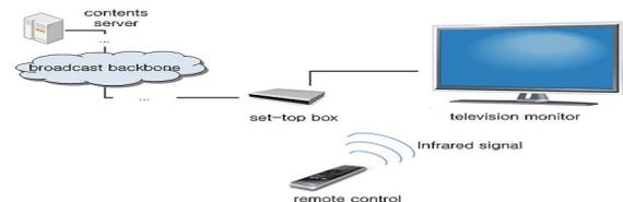
Figure 1. Broadcasting system and set-top-box (STB)
