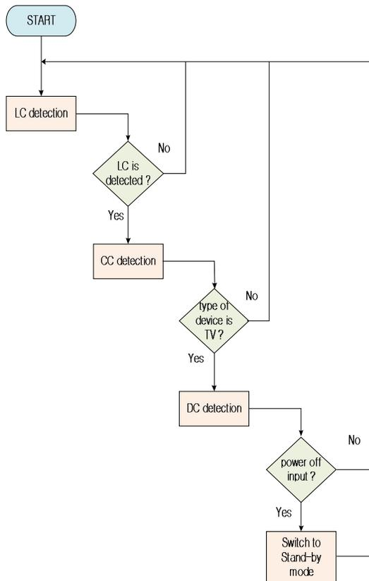
Figure 3 Flowchart of proposed power-saving scheme in STB.
