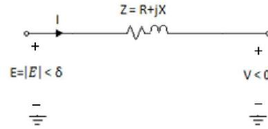
Fig. 1. Basic two-source system with a connecting line.
