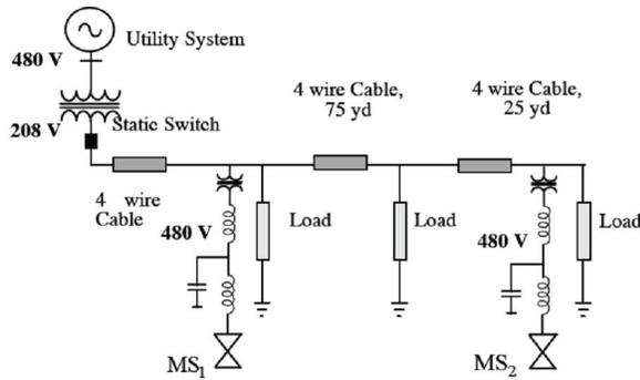
Fig. 4. The Micro-grid under study.
