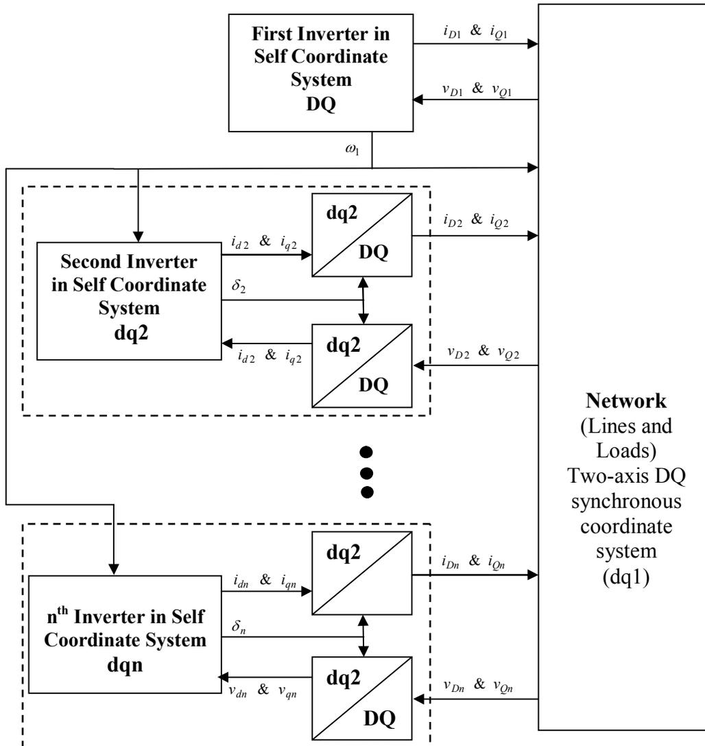
Fig. 3. The parts of Micro-grid and their relationship in view of modeling.
