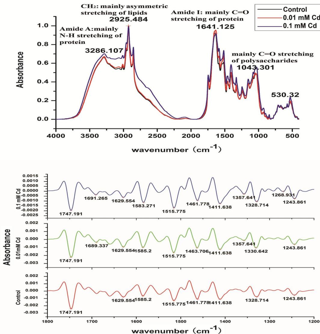
Figure 1. Comparative spectra of control, 0.01 mM Cd and 0.1 mM Cd. Upper: native spectra in the regions of 4000-400  $\text{cm}^{-1}$ ; Under: the second derivative spectra in the regions of 1800-1200  $\text{cm}^{-1}$ . Each curve represents the average spectrum of three individuals.
