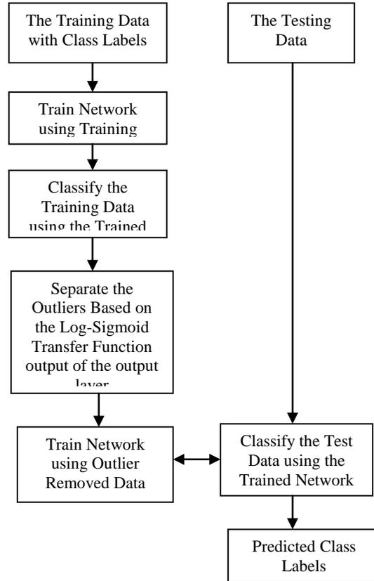
Figure 4. The Outlier Removed Training and Classification Model
