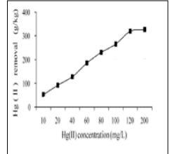
Figure 2. The effect of initial Hg (II) Concentrations on its removal by sewage sludge carbon [9].
