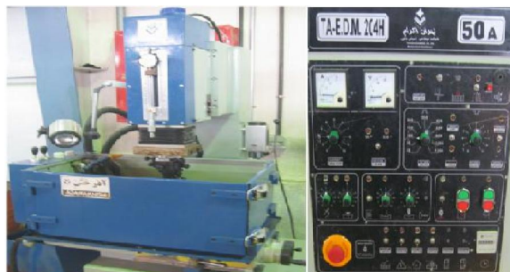
Figure 3. EDM machine (model: 204H)
