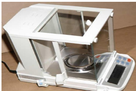
Figure 4. 'AND' balance (model: GR-300) used for weight measurements
