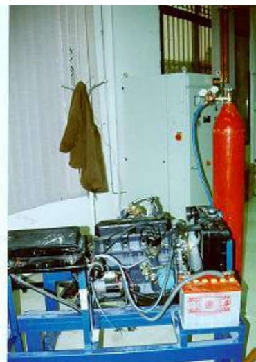
Figure 7 Implement used in 7 Hydrogen – burn of peykan engine project
