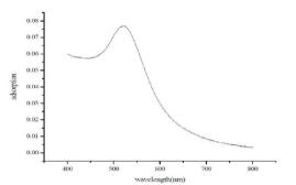
Figure (1) UV-vis spectroscopy of colloids gold nanoparticels
