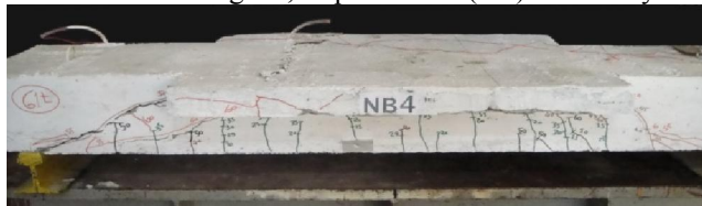
Fig. 7d, Experimental (left) and Analytical (right) crack pattern for Specimen NB4.
