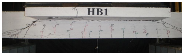
Fig. 8a, Experimental (left) and Analytical (right) crack pattern for Specimen HB1.
