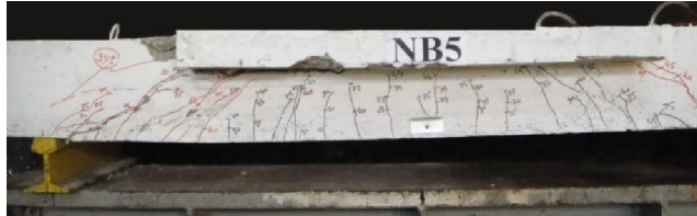
Fig. 7e, Experimental (left) and Analytical (right) crack pattern for Specimen NB5.
