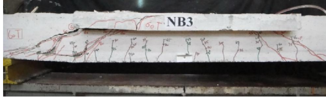
Fig. 7c, Experimental (left) and Analytical (right) crack pattern for Specimen NB3.
