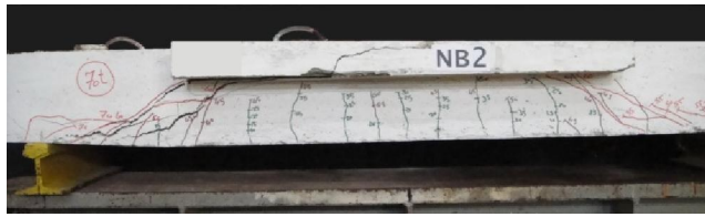
Fig. 7b, Experimental (left) and Analytical (right) crack pattern for Specimen NB2.
