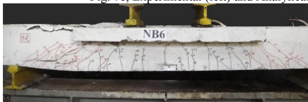
Fig. 7f, Experimental (left) and Analytical (right) crack pattern for Specimen NB6.
