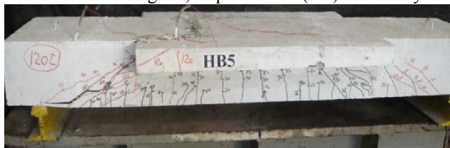
Fig. 8e, Experimental (left) and Analytical (right) crack pattern for Specimen HB5.
