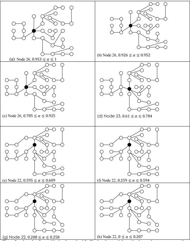
Figure 3: a, b, c, d, e, f, g, and h give the optimal facility locations and the optimal spanning trees representing routing for different values of  $\alpha$
