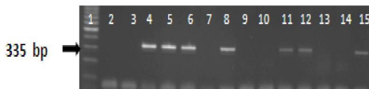
Figure 2: Gel electrophoresis using insert specific primers: lanes 4,5,6,8,11,12,15 show single bands of the insertion fragment of 335 bp so considered ID heterozygote, while lanes 2,3,7,9,10, 13, 14 no bands indicating DD homozygote, lane 1 shows 100 bp marker.
