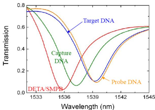
Figure 5. The transmission spectrums of DNA hybridization.
