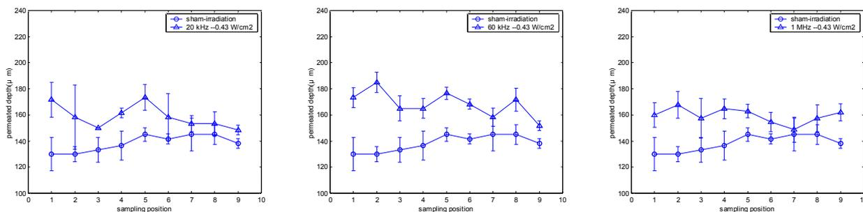
**Figure 6.** The average values of permeated depth as a function of sampling position for the skin sample with exposure frequencies of 20, 60 kHz and 1 MHz: (a) demonstrate the frequency of 20 kHz with intensities  $0.45 \text{ W/cm}^2$ , (b)(c) demonstrate the frequency of 60 kHz and 1 MHz.
