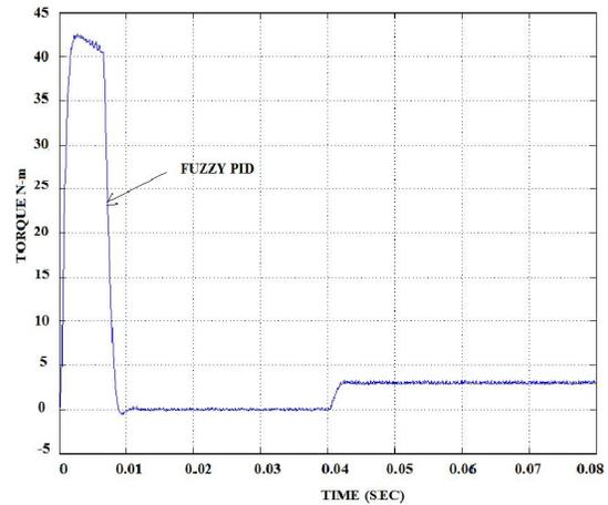
Figure 15 Torque Response of Fuzzy PID Controller
