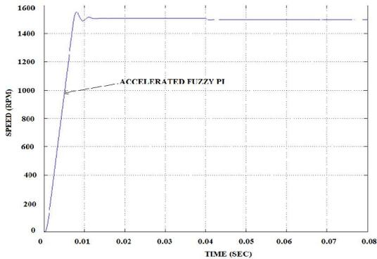
Figure 13 Speed Response of Accelerated Fuzzy PI Controller
