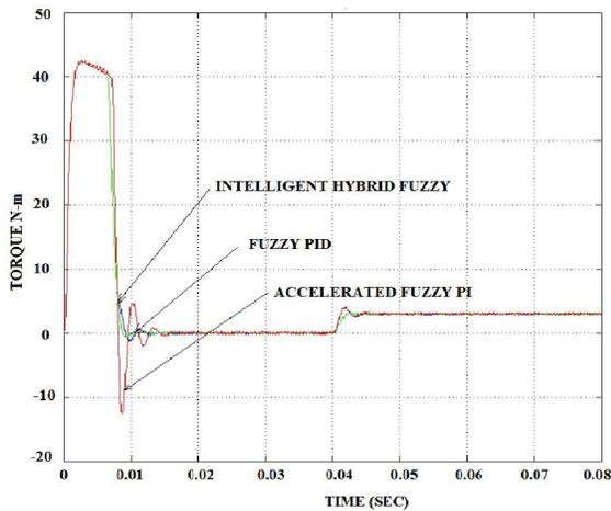
Figure 19 Comparison of Torque Response for Fuzzy PID, Accelerated Fuzzy PI and Intelligent Hybrid Fuzzy Controllers
