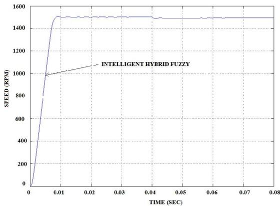
Figure 14 Speed Response of Intelligent Hybrid Fuzzy Controller
