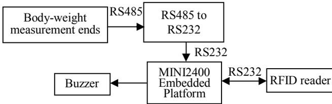
**Figure 6.** Block diagram of body-weight measurement ends.
