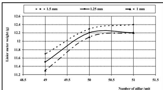
Fig. (14) The relationship between liner meter weight (g/m) and the number of pillar yarns, at inlay tape thickness (20) micron varieties inlay tape width.
