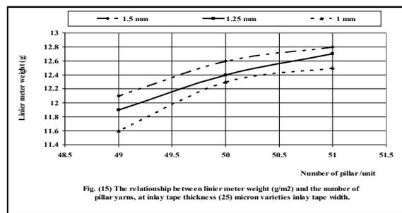
Fig. (15) The relationship between liner meter weight (g/m2) and the number of pillar yarns, at inlay tape thickness (25) micron varieties inlay tape width.
