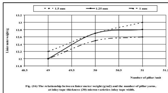
Fig. (16) The relationship between liner meter weight (g/m2) and the number of pillar yarns, at inlay tape thickness (30) micron varieties inlay tape width.
