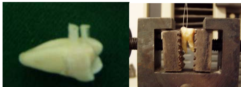
Figure 1: a, specimen with micro-cylinders bonded to buccal surface; b, \mu SBS compartments
