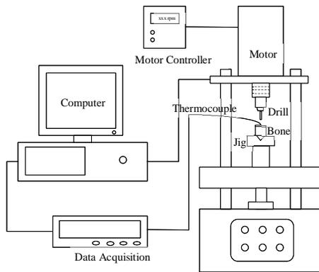
**Figure 1.** Experimental setup for bone temperature rise measurement
