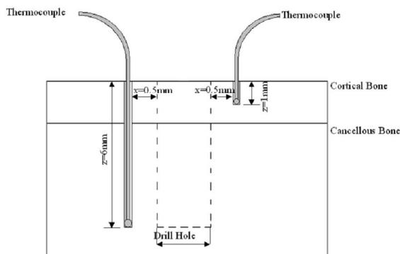
**Figure 2.** Schematic illustration of thermocouple embedded positions
