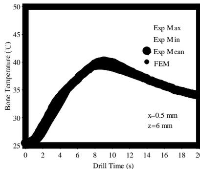
**Figure 6.** Comparison of experimental and numerical results for variation of bone temperature with drilling
