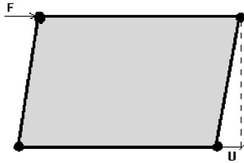
Figure 1. Plate of steel shear wall
