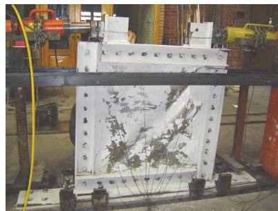
Figure 5. The establishment of the samples in a cyclic experiment completion
