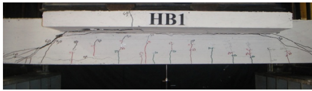
Fig. 8a, Experimental (left) and Analytical (right) crack pattern for Specimen HB1.
