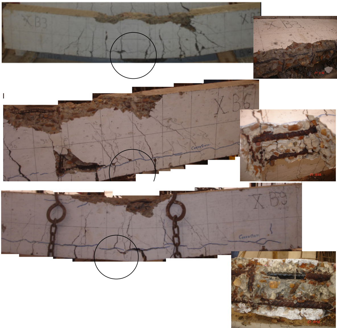
Photo 2. Effect of salt-percentage (s/c) on failure-mode of tested beams at 18 months age.
