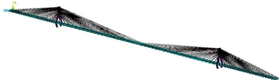
Fig.8. Three-Dimensional Finite Element Model of Tataru Bridge
