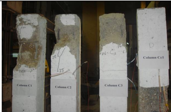
Fig. (8) crack pattern and the shape of failure of c1, c1,c2,c3
