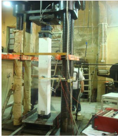
Fig. (6) Set up of loading of the tested columns
