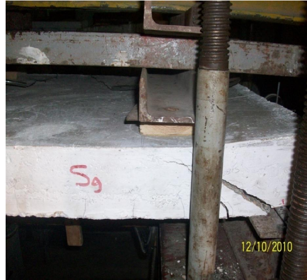
Figure (12): Shear failure of pre-slab S9.
