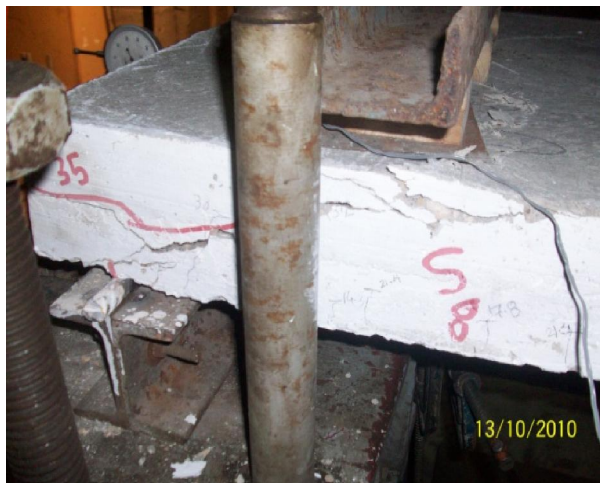
Figure (11): Shear failure of pre-slab S8.
