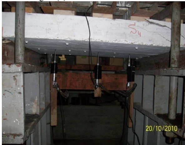
Figure (7): Shear failure of pre-slab S4
