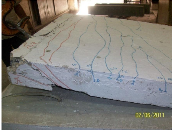
Figure (10): Shear failure of pre-slab S7
