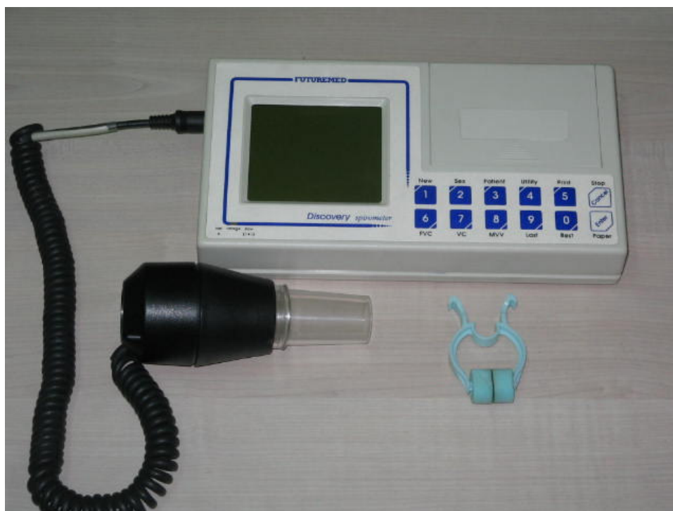
Fig. (1) Futuremed Discovery Hand held Spirometer
