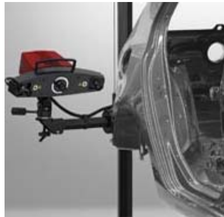
Figure 1. ATOS non-contact laser scanning system
